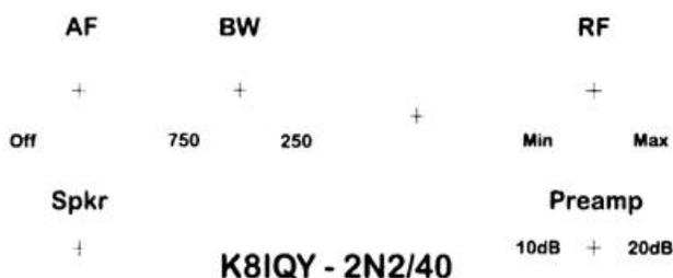
One of the things that probably isn’t obvious, although it is mentioned elsewhere in the article, is that the rig’s On-Off switch is incorporated in the Audio Gain potentiometer. This was a convenient place to add it, and saved finding another place on the already crowded front panel for a power switch. Another item that was mentioned earlier was the ability to switch the RF amplifier to a higher gain. That switch is the one the lower right hand corner labeled Preamp.
