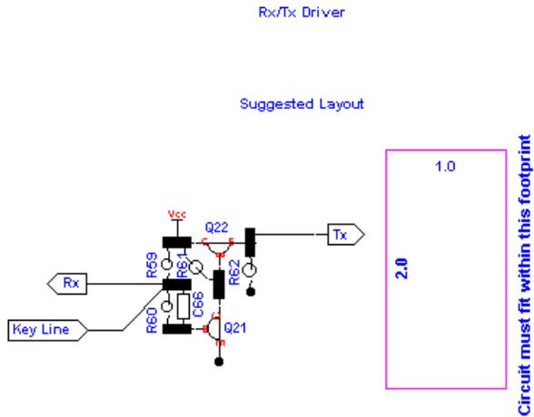
As you can see, this section is really simple-nothing critical in terms of layout, and lots of space to build it. Once it is completed and its port pads are wired to the corresponding port pads in the receiver and transmitter, your 2N2/40 is complete, except for wiring in the controls, jacks, and putting it in a case. Also, don't forget to connect the "A" pads together so the antenna signal can get to the receiver.
