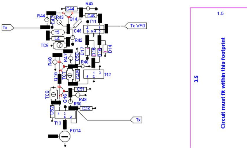
This section should be built from the top down, and right to left. I'd recommend starting with the single balanced mixer and then follow that with the local oscillator. These two sections could almost be done together, since they are adjacent to each other, and tightly integrated.
