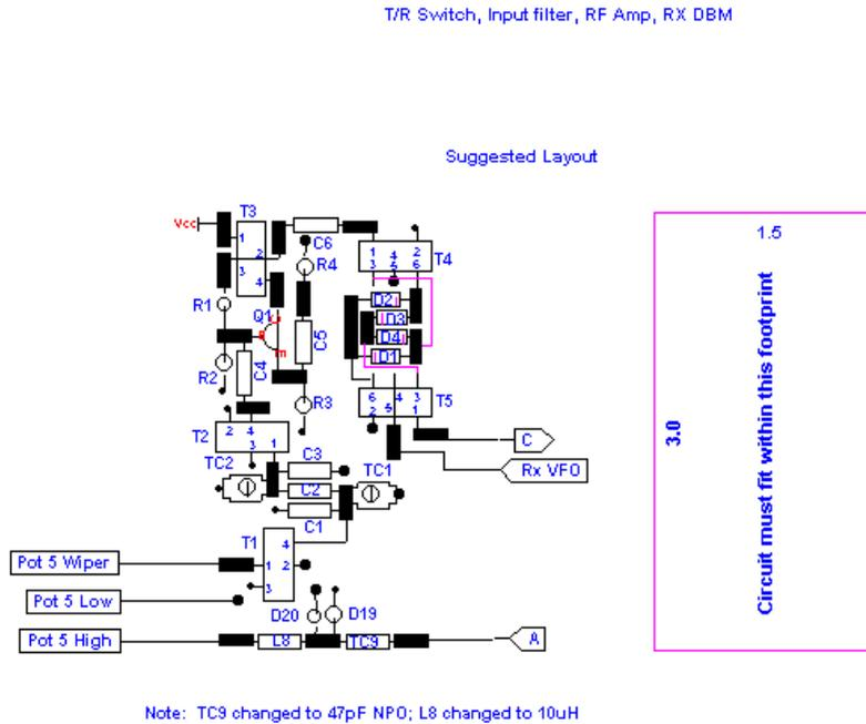
This section should be built from the bottom to the top, and from right to left. Start with the input pad for the T/R switch (Port A) and end with the DBM on the top right. Once this portion is built, it too can be tested, using a general coverage receiver. I'm assuming that you have the VFO built and working correctly and its output is routed to the pad labeled VFO.
